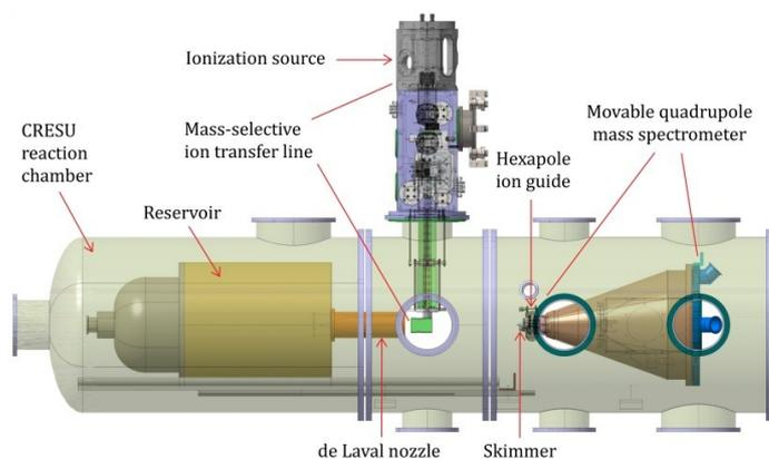
Figure 1: The CRESU reaction chamber incorporating the new mass-selective ion transfer line.
